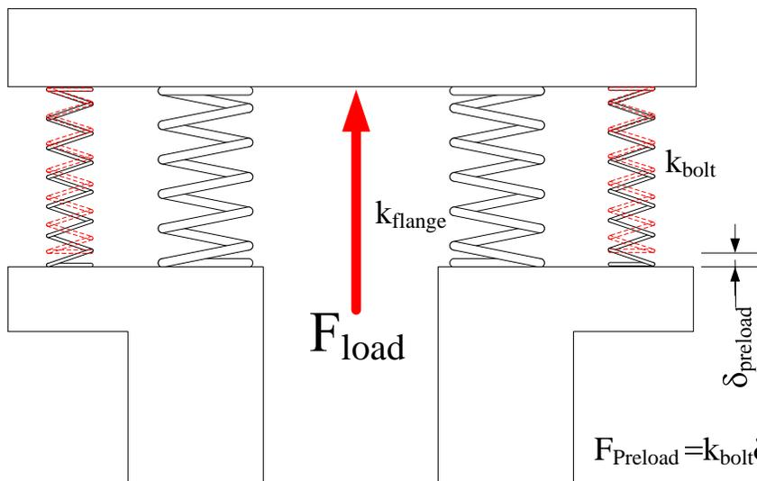
$$F_{Preload} = k_{bolt} \delta_{preload} \quad 9-9$$
