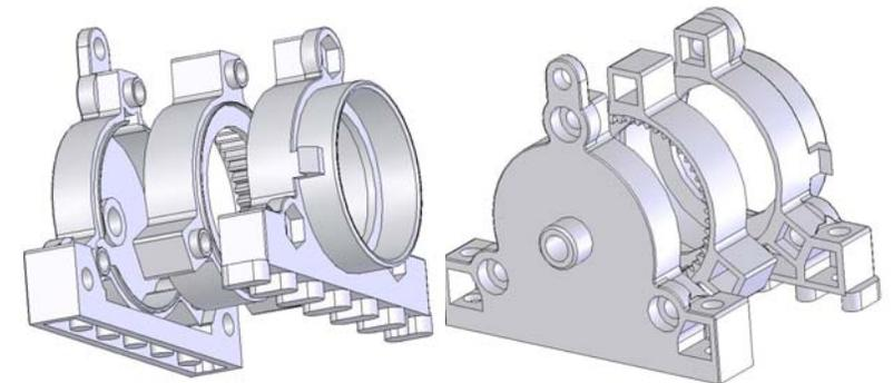
Prof. Slocum, Nevan Hanumara, and Radu Gogoana redesigned the Tamiya planetary gearbox (see Topic 7) to be deterministic with the use of Lego™-like bumps and sockets between stages so they snap together and are precisely aligned via the principle of Elastic Averaging
