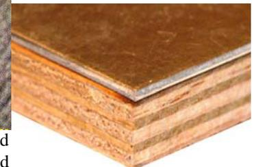
Aluminum epoxied to one side of plywood
